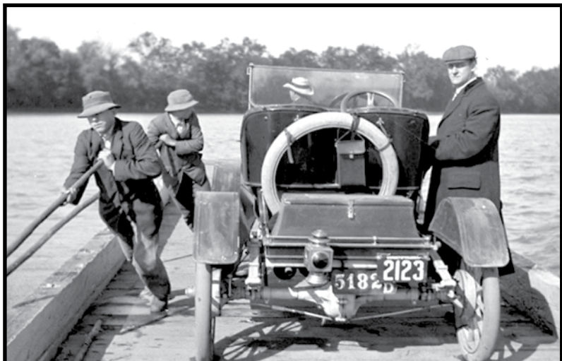
White's Ferry: Crossing the Potomac, October 17, 1909. It appears that the only means of propulsion across the river in this photo was by 'poling'—moving the ferry across the river using long poles to push against the riverbed.
